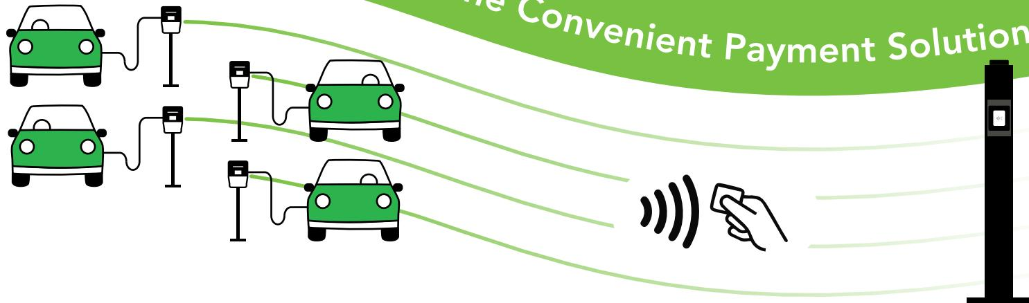
Managing multiple charging points with separate payment terminals is expensive and complex. The Charge-M8 Sigma Payment Kiosk solves this by offering a single, centralised contactless payment solution that supports multiple chargers at once.
