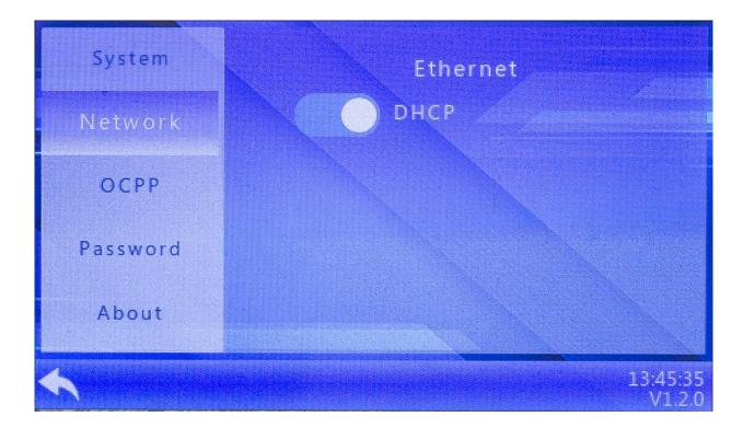
For specific network routes (secure or isolated network routing) unselect the DHCP toggle button which will then open a screen for entry of the IP details provided by the site IT department.
